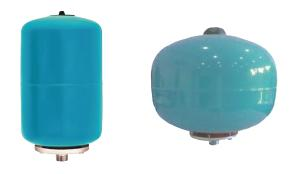
According to directive PED 97/23/CE Replaceable EPDM Membrane Operating Temperature =  $-10^{\circ}C$  /+100°C Precharged Pressure = 3 bar
